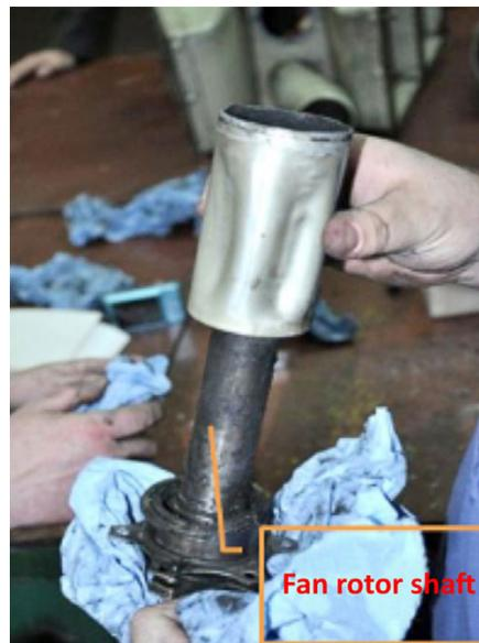
Figure 4. Dents in the outer case
