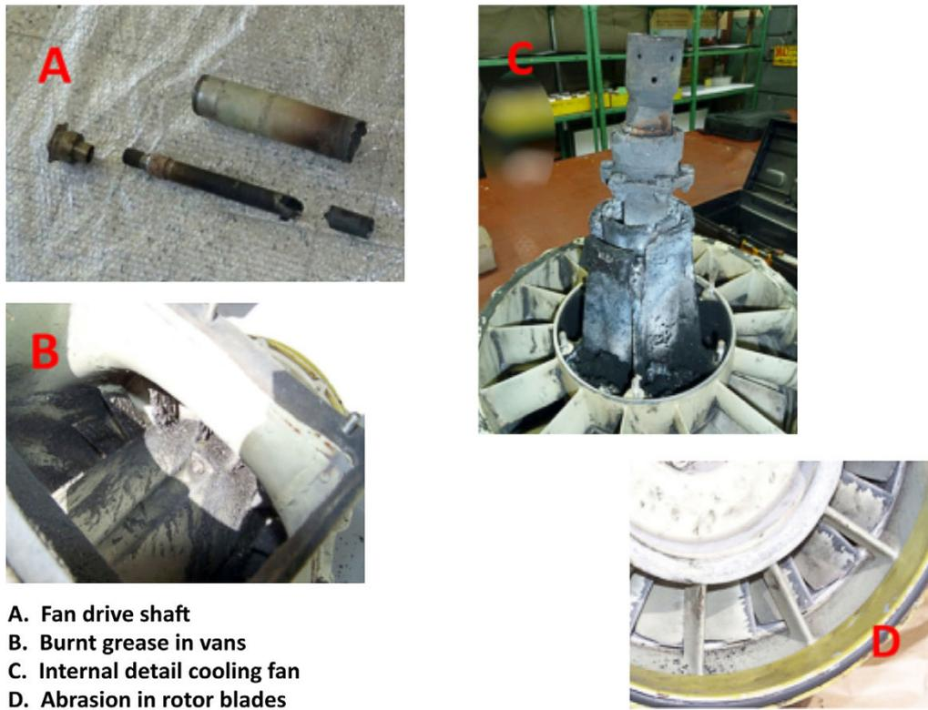
Figure 3. Close-up of the fan components
