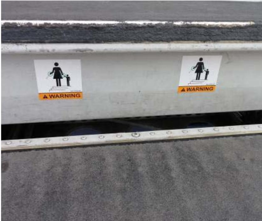
Fig. 4 – Warning signs on the steps. Similar signs are also present inside the aircraft door to be visible to passengers when disembarking.
