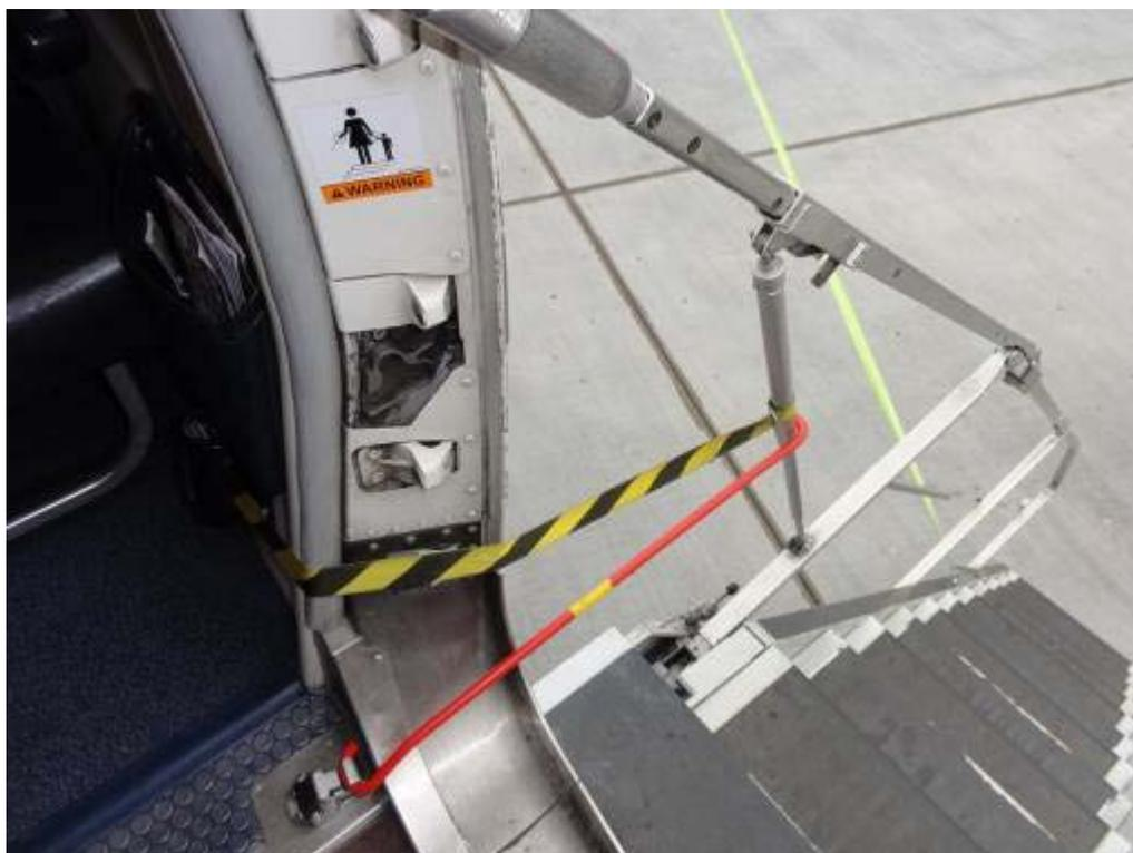
Fig. 3 – The upper part of the aircraft stairs with fall protection installed. Note also the warning sign.
