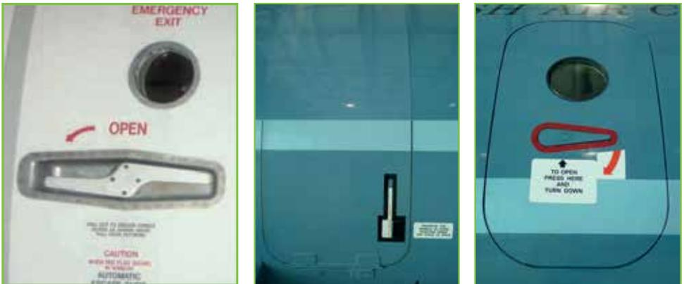
**Example door release mechanisms.**
