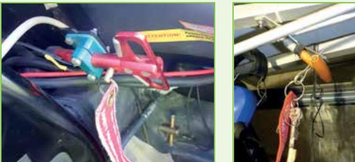
*Example ballistic parachute activation handles (safety pin installed).*
