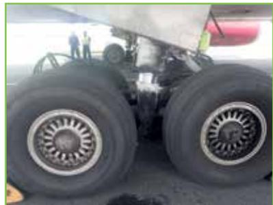
*High pressure aircraft tyres may be damaged during accidents and should be approached with caution.*
