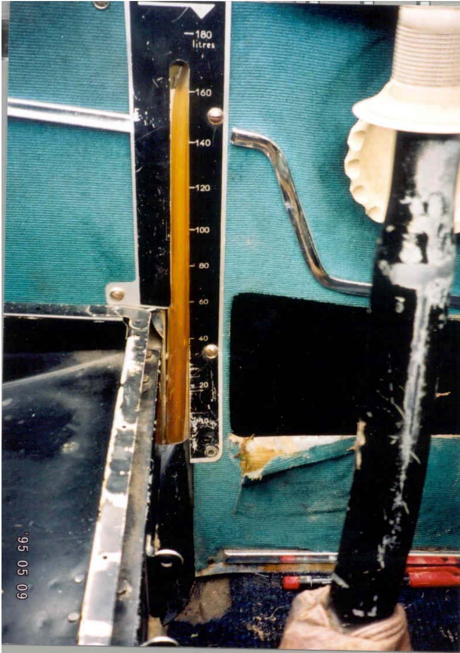
Empty fuel contents gauge, located on cockpit wall, pilot's side, following the forced landing at Ballycorney.
