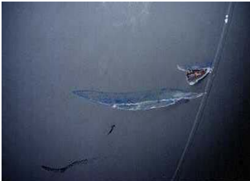
Fig. 1 Damage to Radome of G-MIDH 6cm I----I
