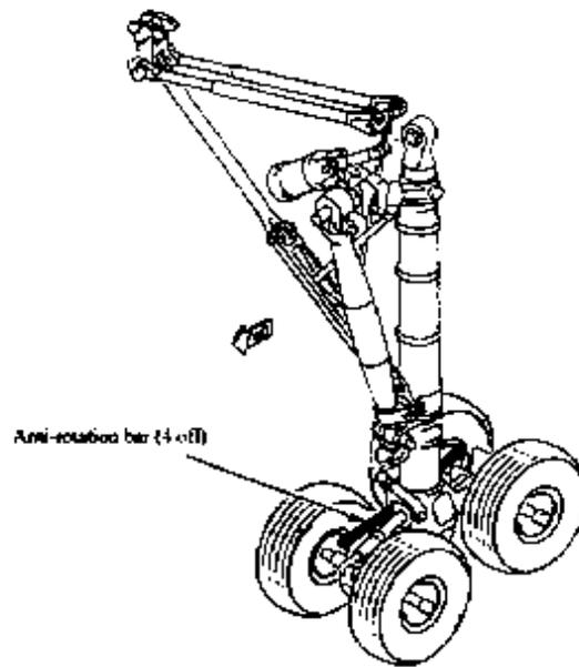
Fig 1 3,500 B4 main landing gear showing arrangement of brake anti-rotation bars.
