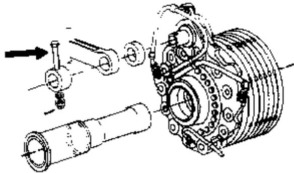
Fig 2 Detail sketch of brake anti-rotation bar retaining collar and bolt (arrowed)
