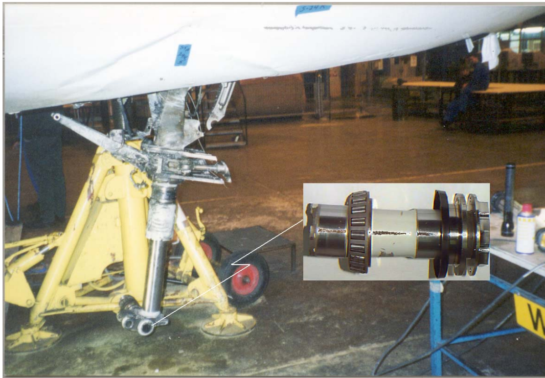
Photo 2. Damage to the drag strut, shock strut and axle of the nose undercarriage assembly and to the nose cone skin of the aircraft. This photo was taken following the removal of the aircraft to the hangar. The damaged nose strut is shown in the normal down position, without its wheels, having been rotated forward from the belly of the aircraft by engineers. Also shown (insert) is the right hand axle, ruptured from the strut, and found in the grass alongside the runway following the accident.
