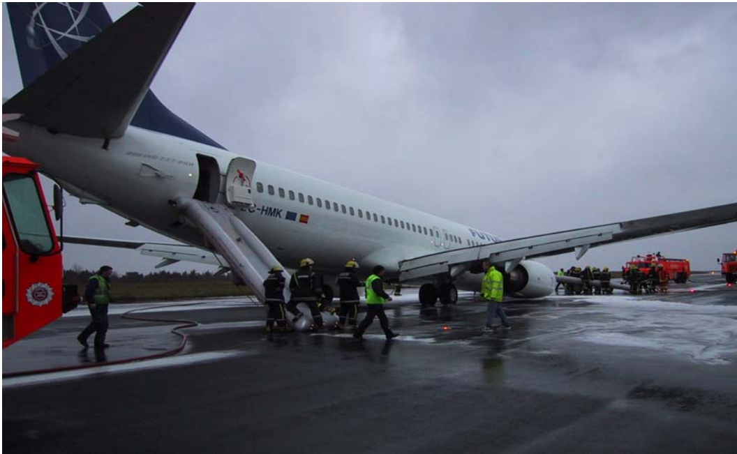
Photo 1. Showing the escape slides deployed on the right hand side of the aircraft
