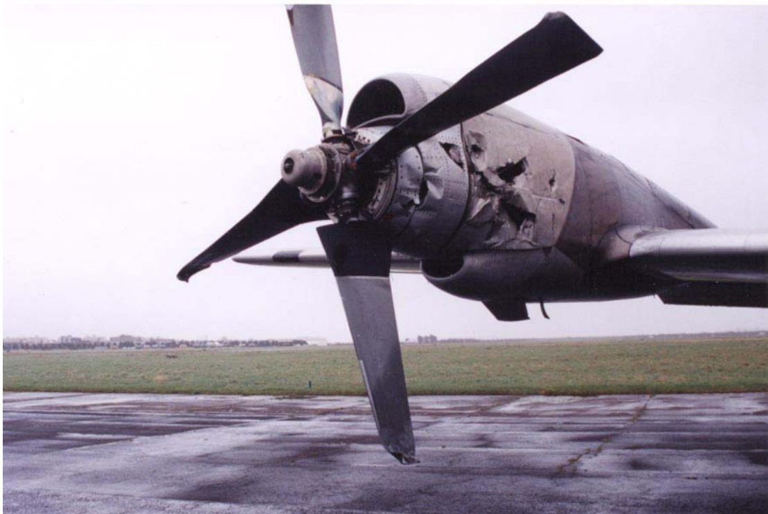
Top – Propeller assembly and part of engine missing from No.3 power plant. Bottom—Damage to No.4 engine inflicted by parts of No.3 propeller
