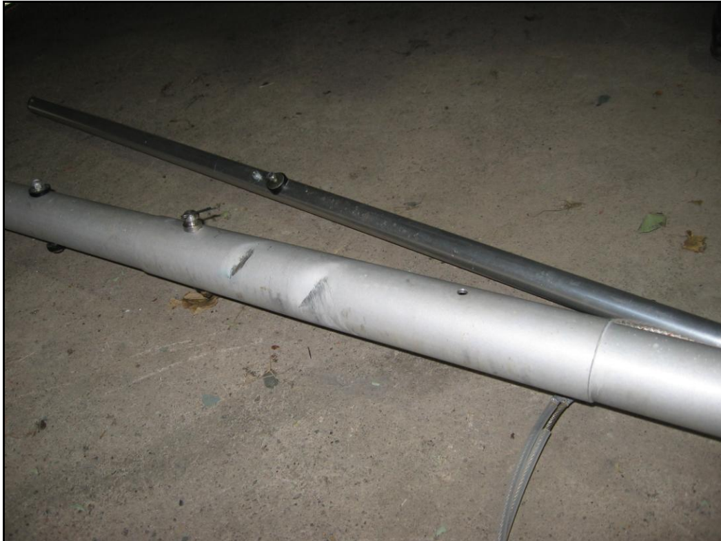
Photo No. 1: Propeller blade strike marks on the keel
