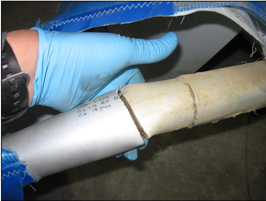
Photo No. 3: Starboard (RH) wing leading edge failure outboard of crossboom, showing inboard part muddy and outboard part clean
