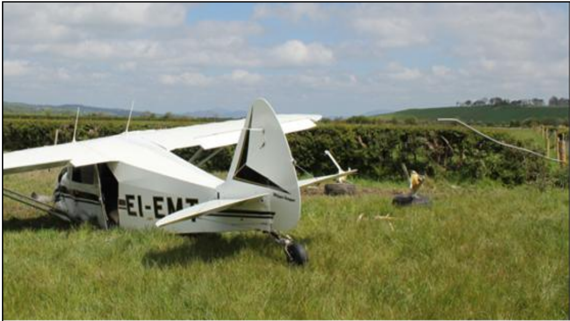
Photo No. 1: Aircraft as it came to rest, note separated wheels and windsock pole
