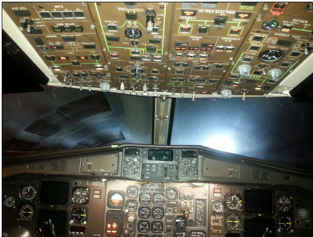
Photo No. 1: Contamination on Windscreen of EI-REI which landed at EICK shortly before EI-REL.
