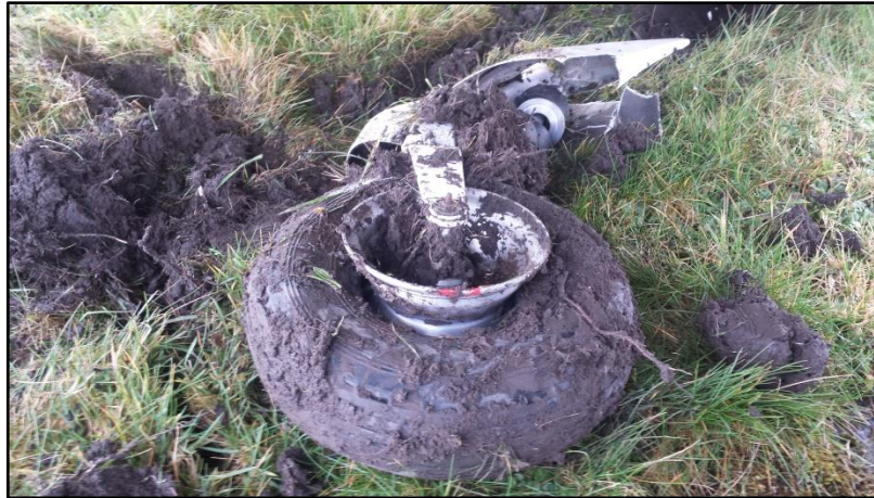
Photo No. 3: Separated nose wheel and deflated tyre.
