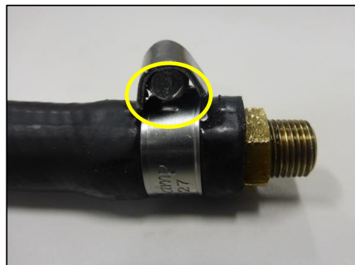
Photo No. 6: Other side of hose clamp/clip showing it to be almost at its minimum diameter.
