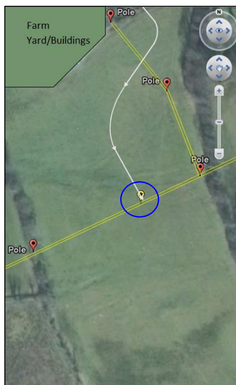
Figure No. 1: Field layout, location of poles (red), overhead wires (yellow), final approach path (white) and site of strike (circled) (adapted from Google Earth )
