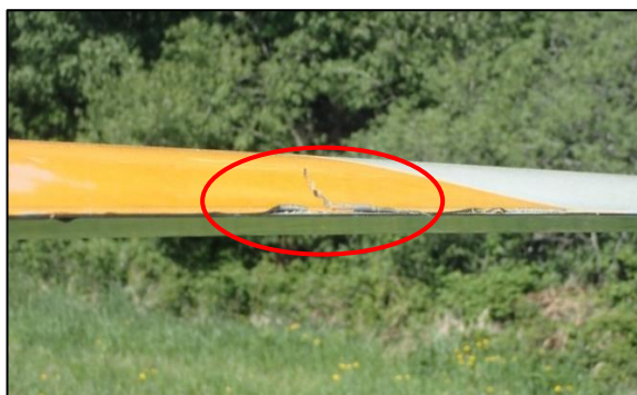
Photo No. 5: Damage to main rotor blade trailing edge
