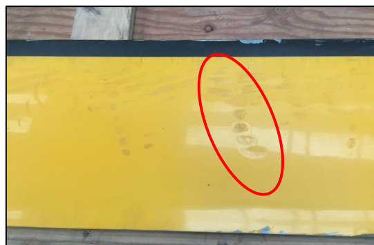
Photo No. 6: Indentation damage to upper surface of main rotor blade
