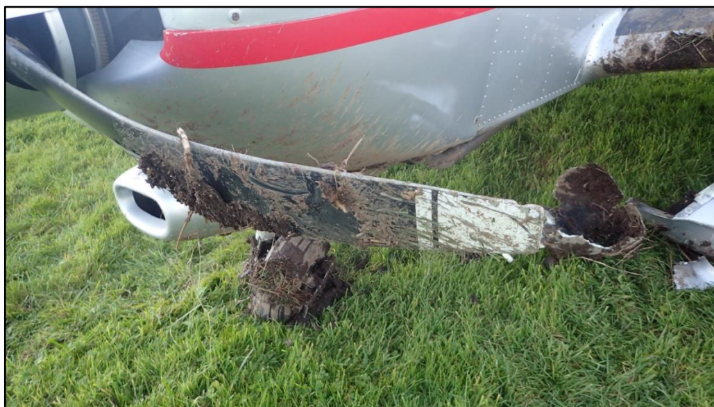
Photo No. 2: Propeller damage suffered during the runway excursion
