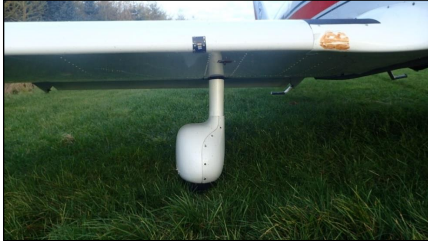
Photo No. 1: Brown witness mark from impact with fence post
