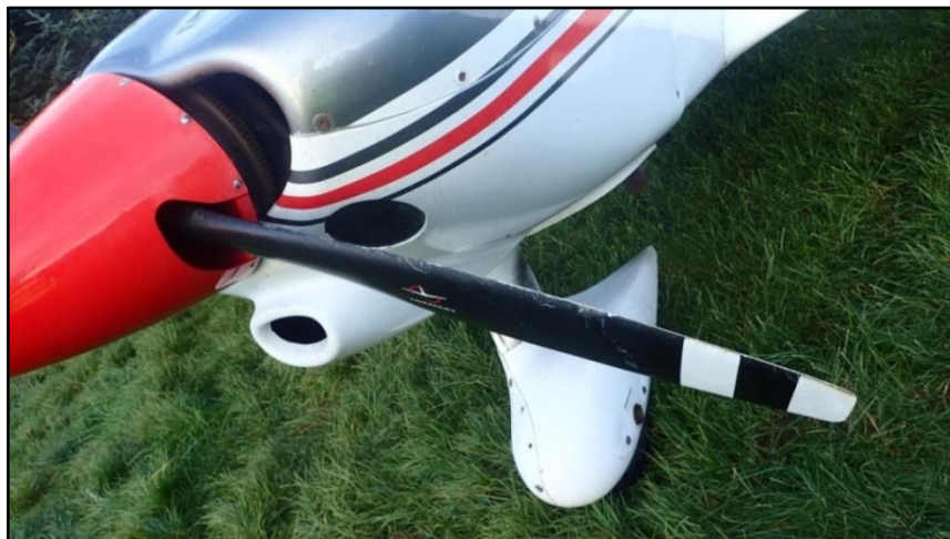
Photo No. 2: Propeller blade exhibiting damage from contact with fence wire
