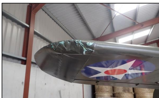
Photo No. 3: Damage to right hand wing tip
