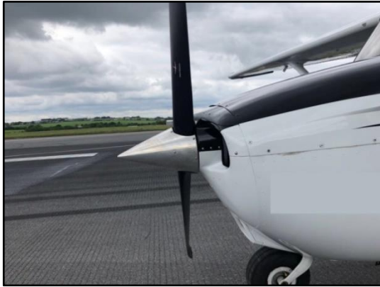
Photo No. 2: The propeller with missing blade tips
