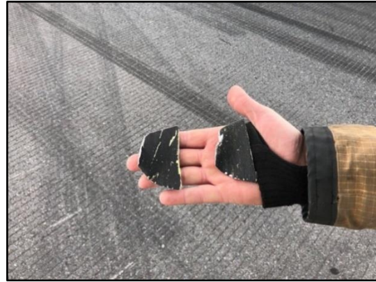
Photo No. 3: The recovered blade tips
