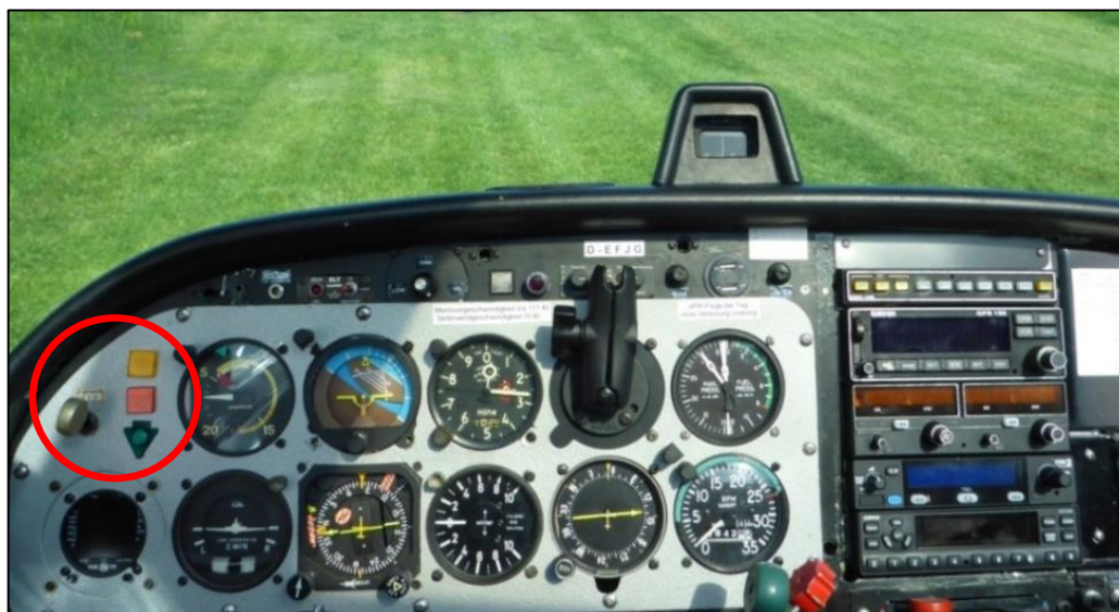
Photo No. 2: Nose landing gear extension/retraction switch and indication lights (circled)
