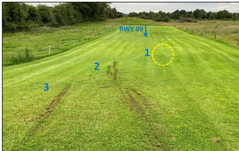
Photo No. 6: Impact marks on RWY 09 (facing west)
