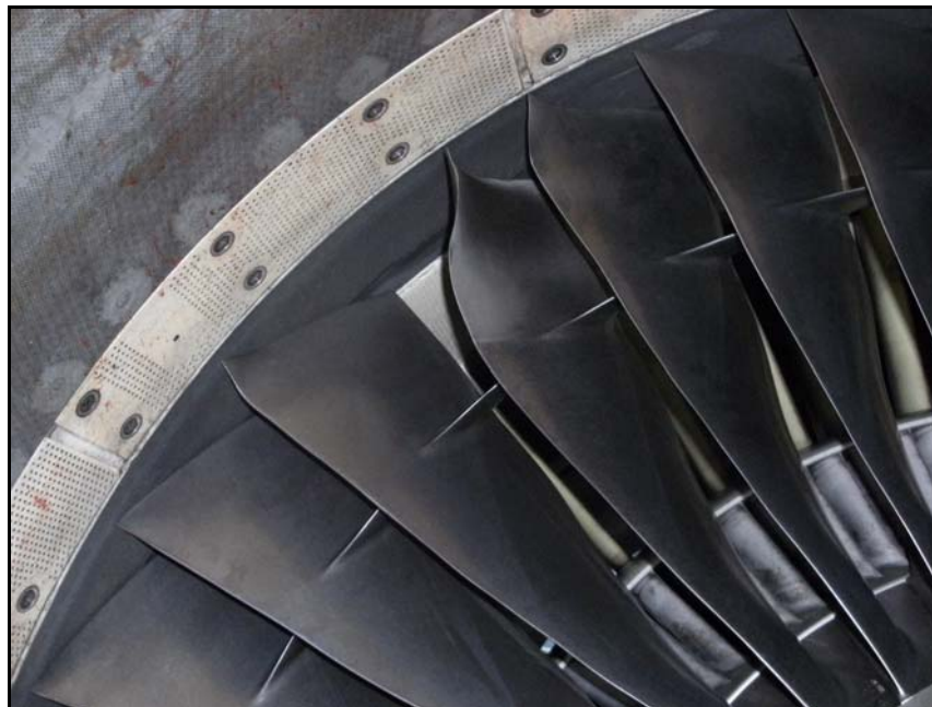
Photo No. 1: No. 1 Engine Fan Blade Damage
