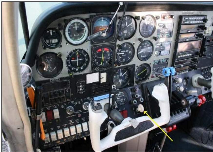
Photo No. 1: Location of Landing Gear Selector
