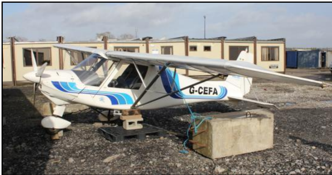
Photo No. 1: G-CEFA with port side main undercarriage assembly removed
